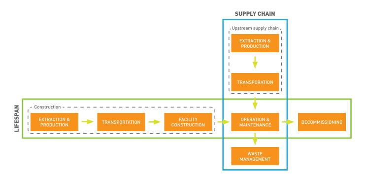
SCHEMATIC OF THE SYSTEMS TO BE CONSIDERED IN A LIFECYCLE STUDY (FROM HATCH, 2014, P. 6)
