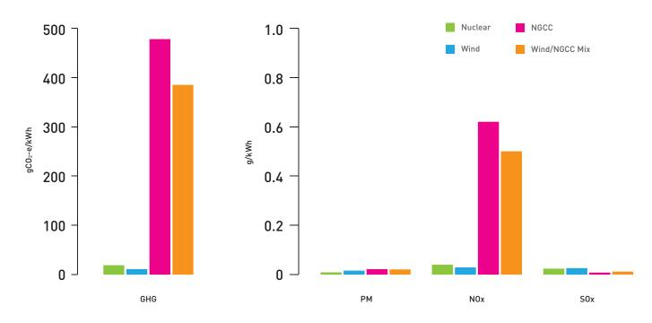
TOTAL LIFECYCLE EMISSIONS OF GREENHOUSE GASES (GHG), PARTICULATE MATTER (PM), NITROGEN OXIDES (NOX) AND SULFUR OXIDES (SOX) FROM POWER GENERATION BY VARIOUS TECHNOLOGIES (FROM HATCH, 2014, P. 47)
